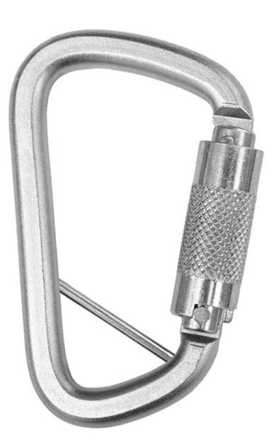
Twistlock captive karabiner with 20 mm gate clearance with a captive bar. 45 kN major axis.
