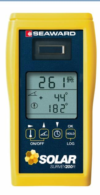
This rugged handheld unit not only measures irradiance, but also has a built-in inclinometer to measure roof pitch, compass to measure roof orientation and thermometer to measure ambient air and module temperature. These unique additional features makes the Solar Survey 200R a truly versatile and indispensable instrument, ensuring optimum conditions for every system installed.
