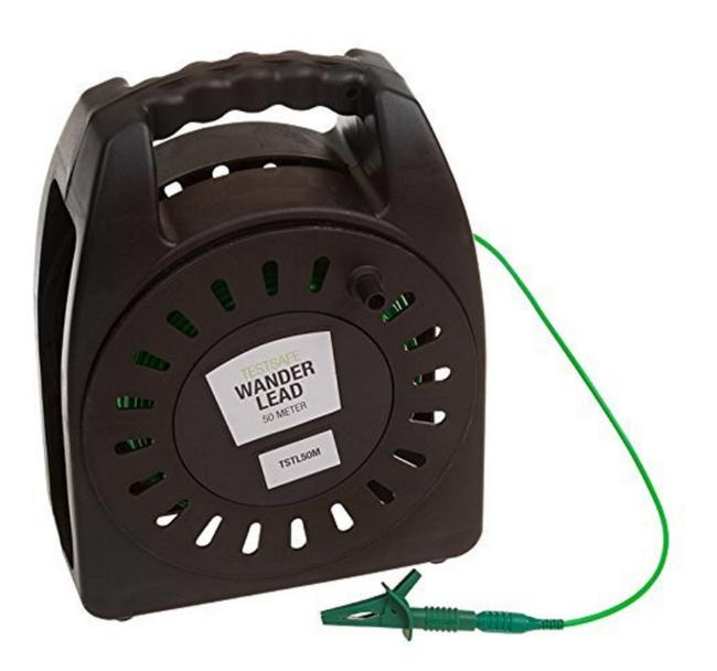
This 50m Wander Lead is suitable for most insulation and multifunction testers providing they use the standard 4mm termination, the lead performs earth bond continuity and R2 measurement where longer wander leads are needed especially for circuit testing of light fittings and ceiling roses.
