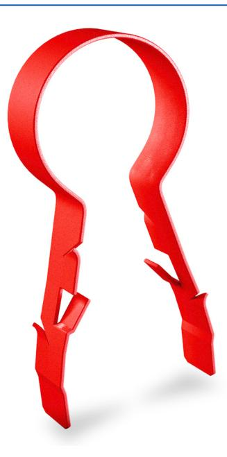
Linian SuperClips<sup>™</sup> are designed specifically for conduit, armoured (SWA) and grouped cables. The cable clips are suitable for all substrates and provide a robust fixing designed to enable significant rotational stress and to support an impressive tensile load of 44kg.
