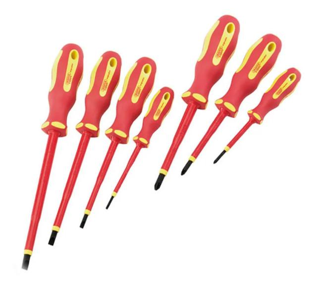
Fully insulated VDE Professional screwdriver Set. Each individual high voltage screwdriver is tested to ensure it fulfils the requirements of EN 60900 legislation. EN 60900 requires all tools to be tested to 10kV, making them suitable for working on live AC circuits of up to 1kV and DC circuits of up to 1.5kV.
