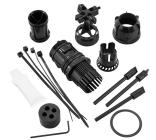
Prysmian Circular Port Entry Glands are used to instal cables into the ports of a joint closure base. The glands are mechanical in nature and are installed onto the cable, then simply pushed into the base of the joint.
