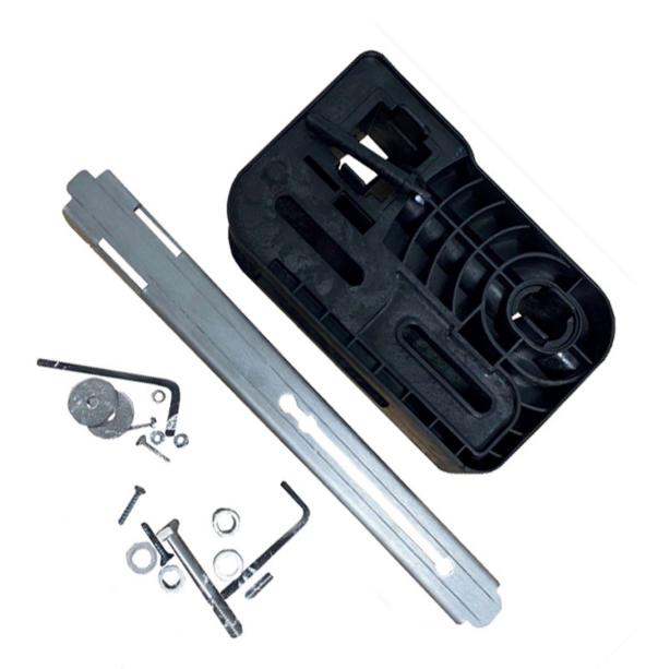
The Prysmian CBT Half Size MOBRA Mounting Kit is fitted to the back plate of the closure. It is then used to mount the closure in a footway box and allows storage in the horizontal and can be pivoted in to a vertical position.
