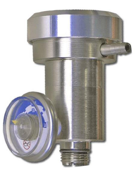
The REG-DF-1 is a C-10 (male thread) demand flow regulator from Honeywell Analytics with a maximum output capacity of 3 litres per minute, so it can be used to calibrate up to 8 docking modules simultaneously.
