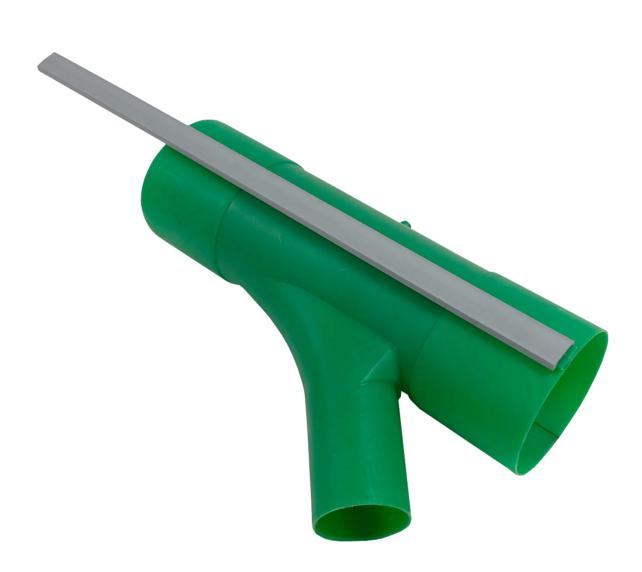
Split swept tee for use with PVC duct system, tees off at 45 degrees from a 96.5mm OD / 90mm ID duct to a 53.9mm OD / 50mm ID swept exit. Hinged for retrospective fitting.
