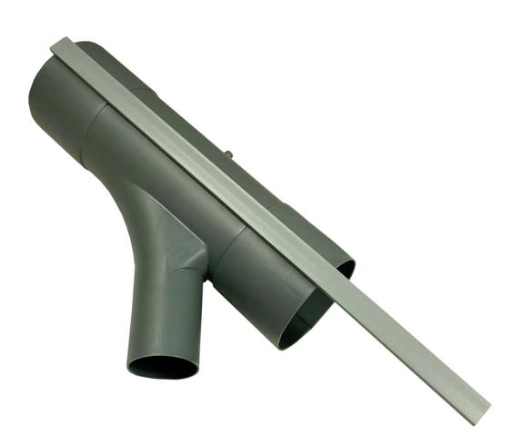
Split swept tee for use with PVC duct system, tees off at 45 degrees from a 96.5mm OD / 90mm ID duct to a 53.9mm OD / 50mm ID swept exit. Hinged for retrospective fitting.
