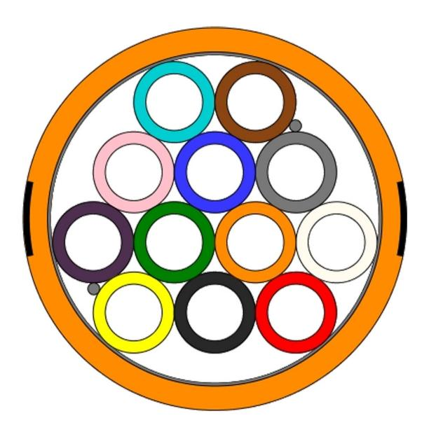
Assembly of PE tubes 5mm OD, each with low friction performance.
