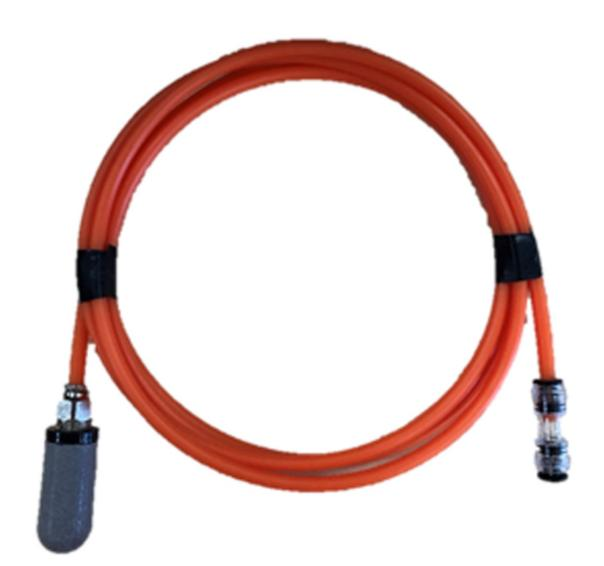
An air stone fibre catcher connected to a 2.4 metre length of 8/4mm microduct with an 8mm straight connector. During blown fibre installations, the air stone allows air to escape via very small pores to prevent air build up within the installation route.
