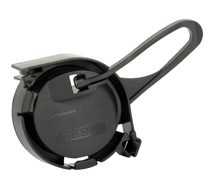
The drop wire clamp is used for the dead-ending of 4mm to 6mm aerial round drop cables distribution networks where spans should not exceed 70m.
