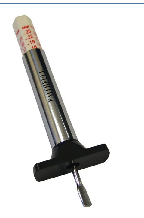
This easy-to-use Tread Depth Gauge quickly checks whether tyres are legal and roadworthy and helps to spot uneven thread wear and tracking errors. It gives fast and easy to read measurement of tyre tread depth from 1 to 24mm in one millimetre graduations on sliding barrel. It has a steel body with easy read sliding plastic centre column.
