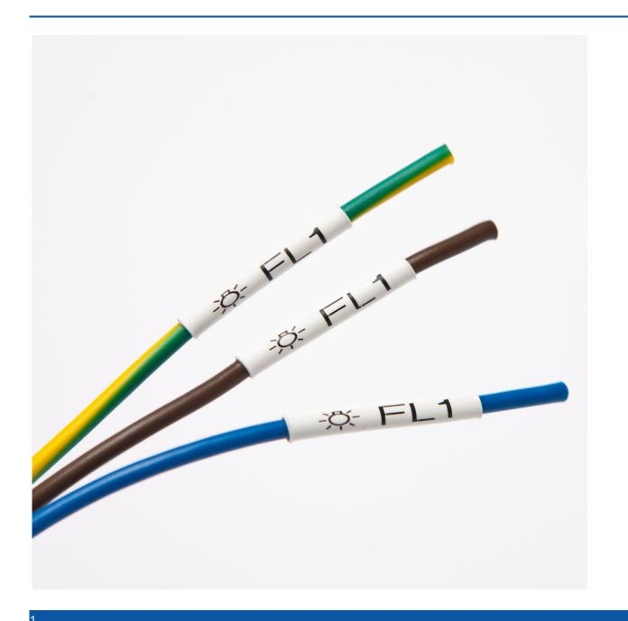
This 23.6mm HSe-251 heat shrink tube tape is designed specifically for permanently marking and identifying cables and wires. With a shrink ratio of 2:1, the HSe-251 black on white tape is recommended for use with cables between 7.3mm and 14.3mm in diameter. Compatible with P-touch label printers that show the HS or HSe logo on the tape cassette cover.
