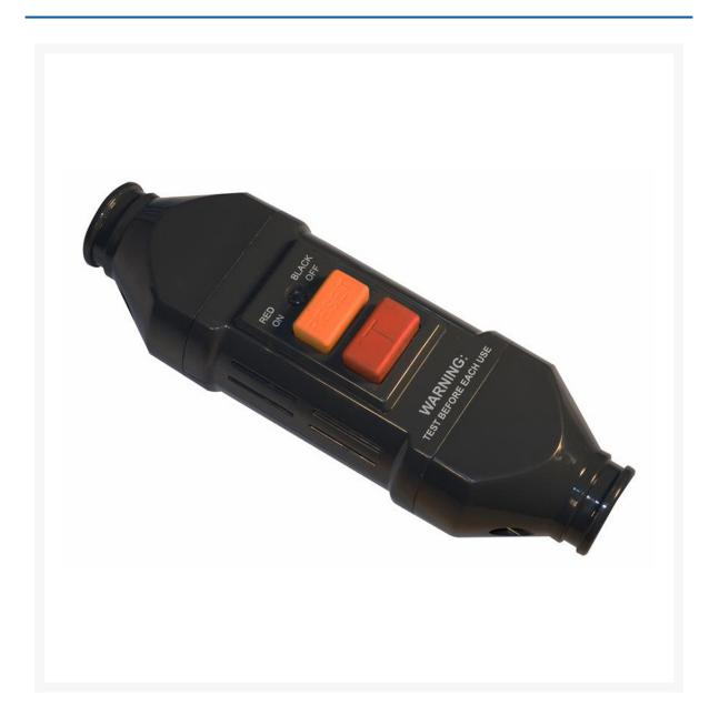
The Masterplug Safety in-line RCD continuously monitors the power supply to an electrical appliance and cuts off the power within 40 milliseconds if an earth current fault is detected. This is fast enough to prevent a fatal electrical shock.
