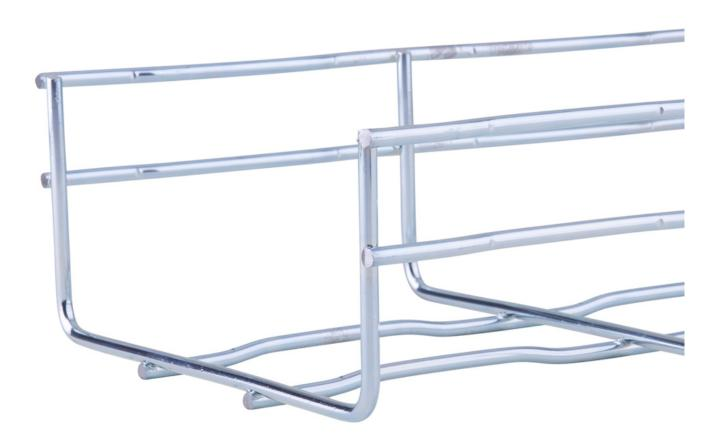
Manufactured from high strength electro zinc plated steel wire, Vergokan steel basket is fast and easy to install using tool-less quick couplers to join lengths of basket.
