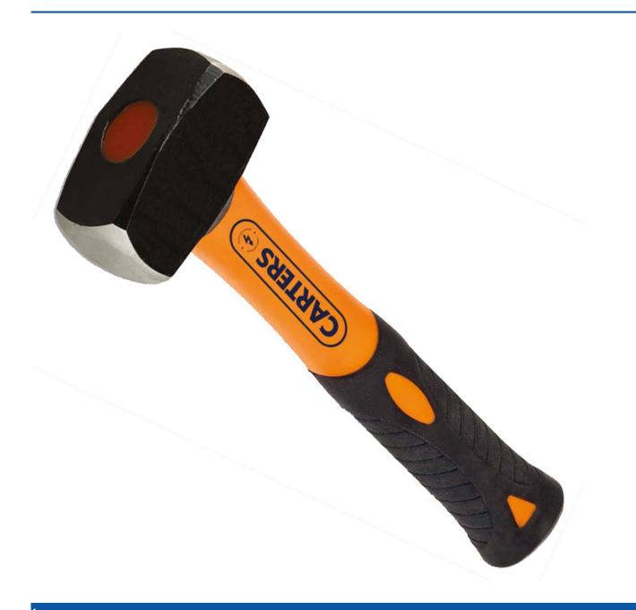
4lb / 1815g lump hammer with a 10" Shocksafe fibreglass shaft and manufactured to the exacting specifications of BS8020:2012, for live working.
