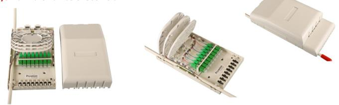
The PBI-8SC is a riser box designed for use within apartment blocks and mid/high rise office blocks. The unit houses three splice trays and up to 8 SC type pigtails and adapters. Each splice tray is able to accommodate 12 fibre splices. An in-line cable entry port enables the box to be installed onto an in-line riser cable and up to 24 drop ports are available for drop cables of up to 5mm in diameter.
