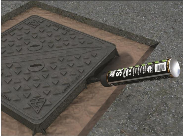
11.12 Ultracrete Instant Road Repair is applied to a depth of approximately 45 mm and compacted to 30 mm (see Figure 7).
