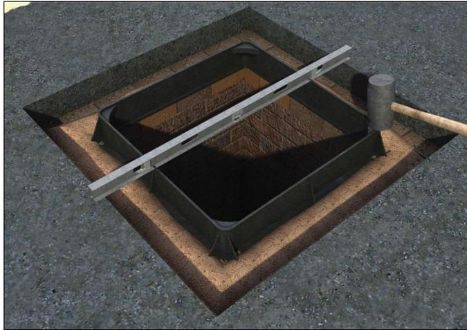
11.7 Any holes within the frame are infilled and the flanges of the frame enveloped by a minimum thickness of 10 mm of the bedding material.
