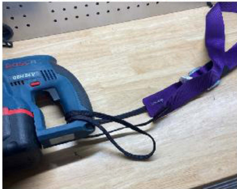
Pull the black webbing through there's no drill handle if no lanyard slot in the drill and create a loop, repeat process as above
