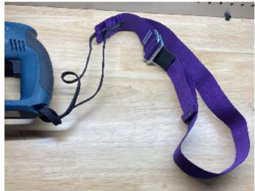
Pull Purple strap completely through the loop to choke the drill bandolier in position
