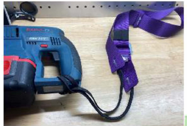
Pull Purple strap completely through the loop to choke the drill bandolier in position
