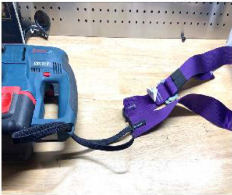
Pull the black webbing through lanyard slot and create a loop
