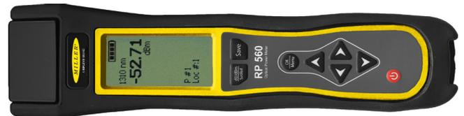
The RP560 allows for either streaming readings testing or saving then offloading of readings. It supports 850, 1300 ,1310,1490,1550,1611, and 1625nm wavelengths as well as 270Hz, 330Hz, 1kHz,and 2kHz tone detection. The RP560 is only available wired on the VIS300C however can be used on other platforms with bluetooth.
