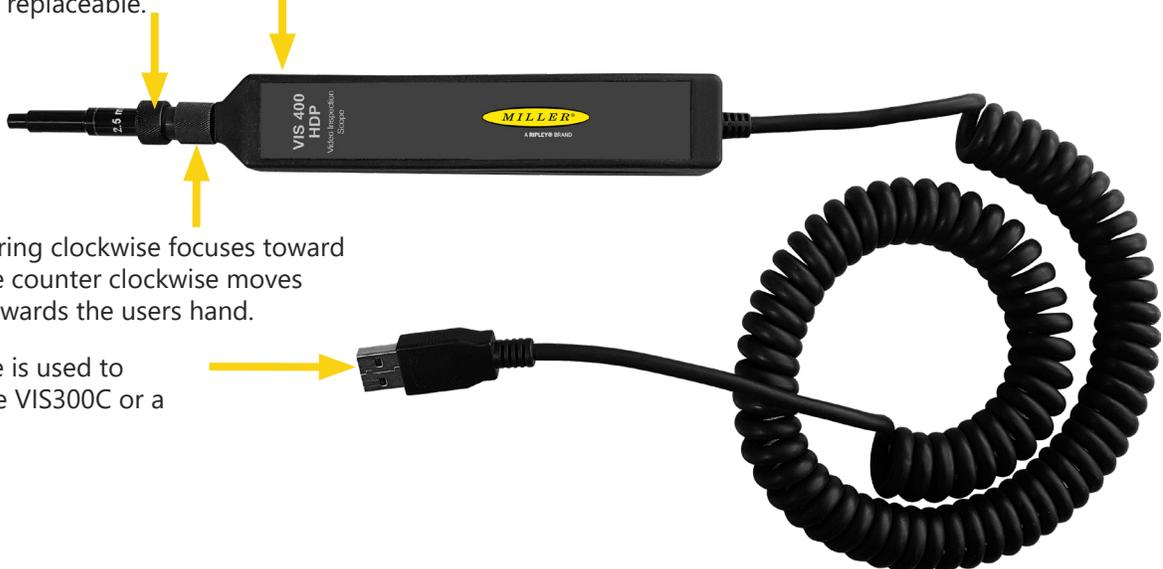
To connect the VIS400 to the VIS300C simply navigate to the home page and plug the USB cable into the side of the unit. Once plugged in the VIS300C will detect the probe and begin showing a live view of the scope.
