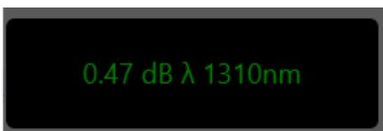
Any readings which fall between the Min and Max values will be displayed in green in the display and the saved data field. Readings which fall outside this range will be displayed in red.
