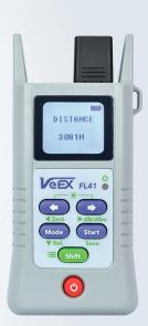
The FL41 is a budget friendly and palm-sized Fault Locator/ Optical Power Meter for measuring fiber spans from 10 m up to 20 km in length. The FL41f has a built-in filter for in-service fault locating. The FL41 is the perfect tool for service activation technicians who need to measure short fiber links and drop fiber for PON, 5G rollout, FTTx, LAN/WAN, and CATV.
