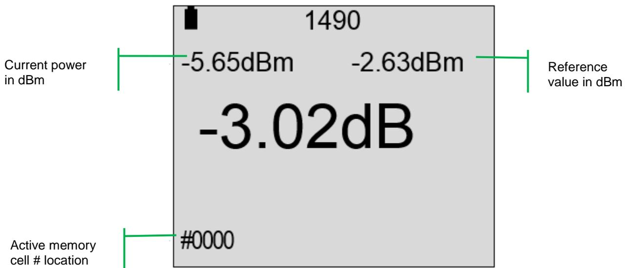
The larger digits represent the relative optical power level in dB (i.e. the loss of the device or fiber under test).
