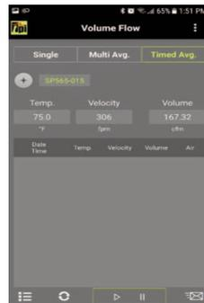
11. When the duct has been completely traversed and prior to pulling the probe out of the last test hole, press the “Stop” icon.
