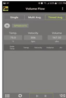
12. The stored reading is the average Temperature, Velocity, and Volume during the timed test.
