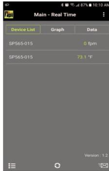
Displays the measured air velocity and temperature.
