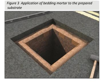
11.2 When packing materials are used to support and level the frame, they must be compatible with the bedding mortar to be used. The Certificate holder can advise on suitable materials.
