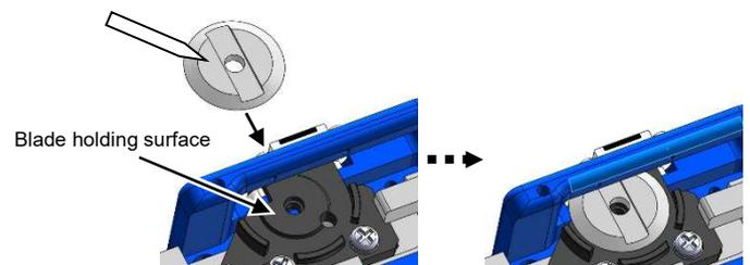
7: Re-insert the gear wheel back in the cleaver following the slotted part of the blade. Align the hole of the gear wheel with the hole of the blade.
