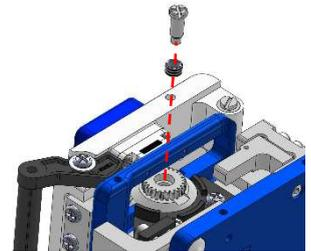
5: Remove the gear wheel and blade.
