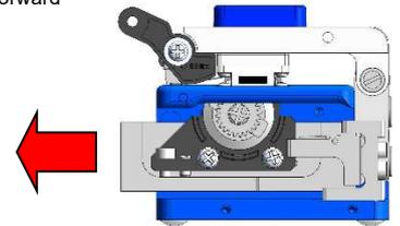
4: Lay the cleaver on its side. Remove the blade setscrew and spring.
