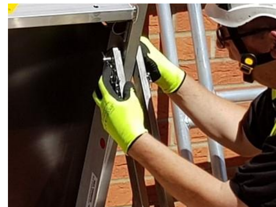
4. Release the dec struts from their parked position and raise to either side of the Dec as shown. Again, with pin from the outside in attach the struts to the Dec frame, R'clips should be inserted to midway position as shown
