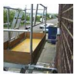
Stand-Off Kit: Allows safe access over deep soffits. The kit comprises a pair of 20cm Stand-Off arms which safely position the platform away from the building
