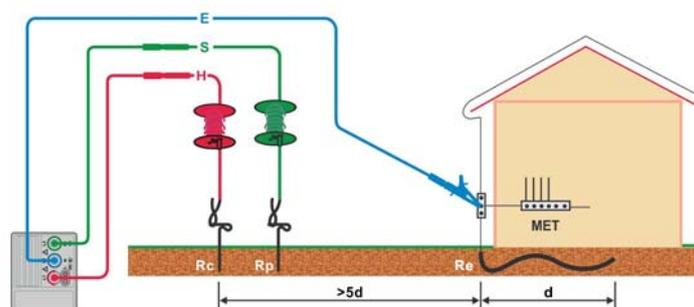
Figure 5.38: Resistance to earth, using extension leads
