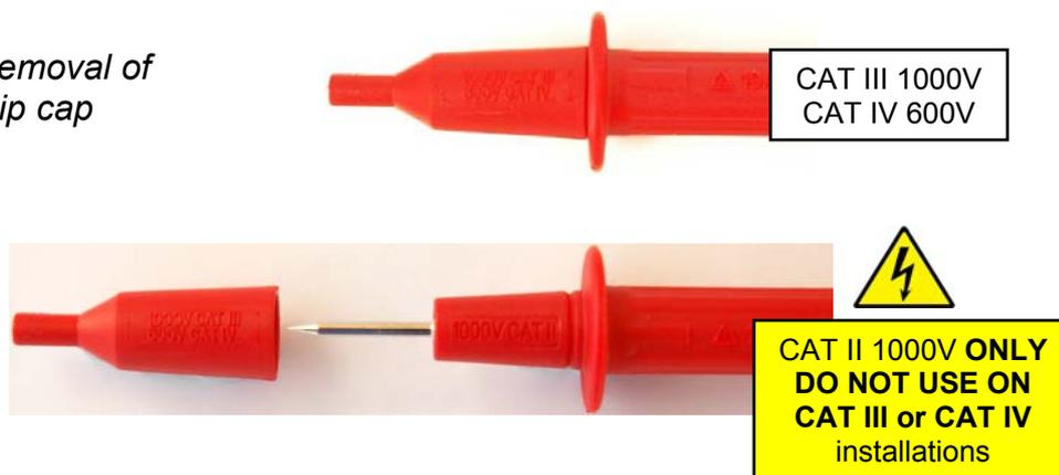
If crocodile clips are to be used, remove the test probe, if fitted, from the 4mm plug by pulling it forward, then push the crocodile clip onto the 4mm plug.
