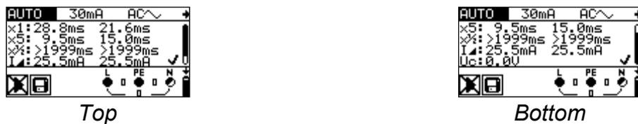
Figure 5.26: Two parts of result field in RCD autotest
