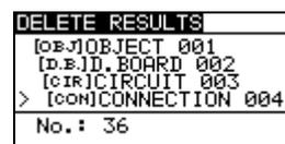
Figure 6.8: Clear measurements menu (data structure field selected)
