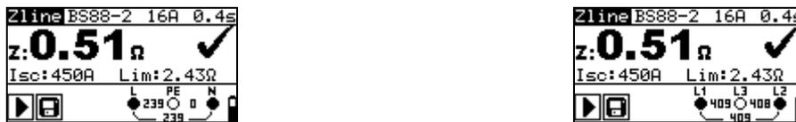
Figure 5.33: Examples of line impedance measurement result
