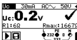
Figure 5.22: Example of contact voltage measurement results
