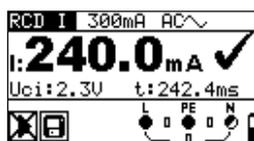
Figure 5.24: Trip-out current measurement result example
