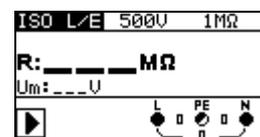
Figure 5.5: Insulation resistance
