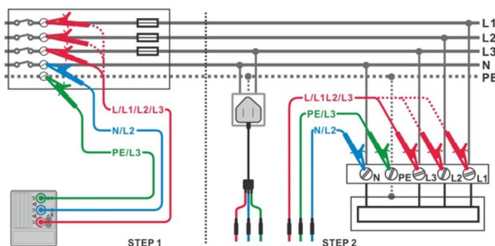
Figure 5.34: Phase-neutral or phase-phase voltage drop measurement
