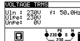
Figure 5.1: Voltage in a single phase system
