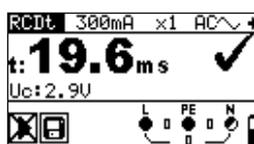
Figure 5.23: Example of trip-out time measurement results
