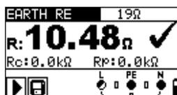
Figure 5.39: Example of earth resistance measurement result
