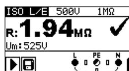
Figure 5.7: Example of insulation resistance measurement result
