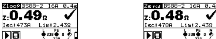
Figure 5.29: Examples of loop impedance measurement result
