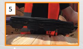
Place a cable tie over each of the tabs and pull hand tight. (Tools not required).
