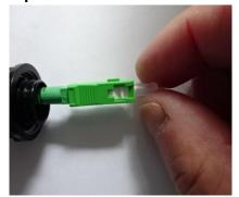
Remove the SC connector protective shroud.
