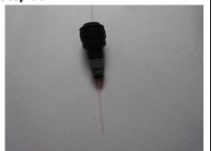
Pass the optical fibre through the 6mm - 3mm connector.
