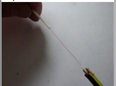
Remove the final section of the loose tube.
