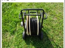
At the CBT Terminal fit the Drop Cable drum into a suitable cable dispenser.
