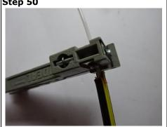
Apply a circumferential cut to the loose tube at the cable butt
