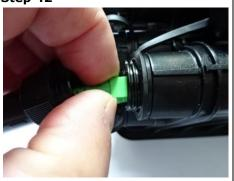
Push SC connector into the adapter. Ensure locating the rib is facing upwards to line on top of the port.
