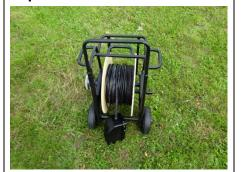
At the CBT Terminal fit the cable into a suitable cable dispenser.
