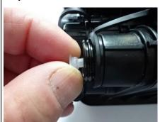
Remove the adapter blanking plug.
