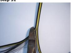
Carefully cut the two halves of the cable sheath, non-mettalic yarns and the steel wire strength members.
