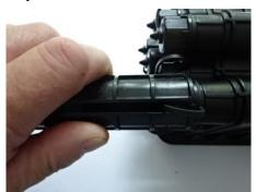
Using the supplied tool remove the cap from the relevant port on the CBT. There is a number by the port for identification.
