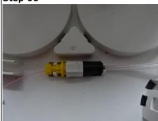
Fit the connector into the locking clips.
