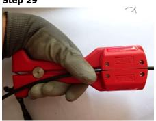
Pull the cutter along the cable.
