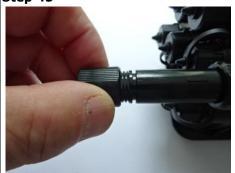
Tighten the clamp nut ensuring the seal is in the end of the shroud.
