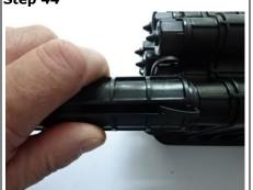
Tighten the shroud nut fully.
