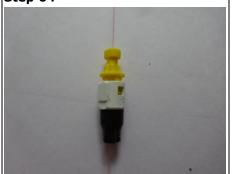
Pass the optical fibre through the connector
