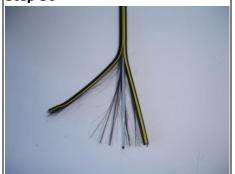
Separate the two halves of the Fibre Drop Cable sheath back to the mark made in step 25.
