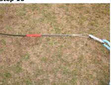
Attach the swivel to the cable using that cable stocking grip.
