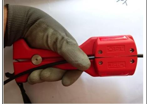
Pull the cutter along the cable.
