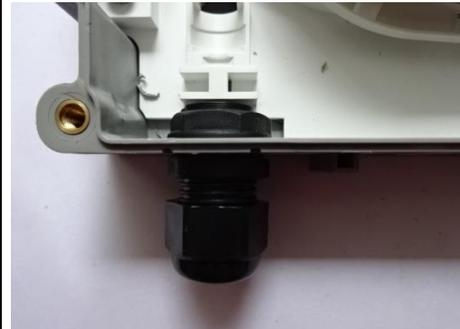
Fit 'O' Seal onto the cable gland and into annular recess in hexagonal face. Push the cable gland into port so that the 'O' Seal sits against outside face of base. Fit Locknut and tighten against inside face of base to secure it.
