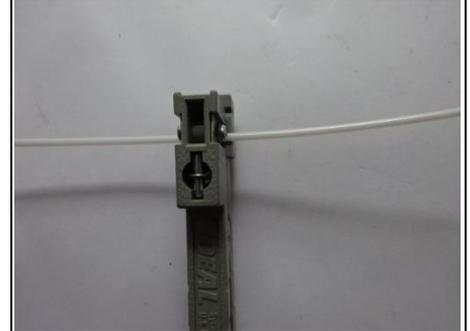
Apply a circumferential cut to the loose tube at 1m from the end of the tube.
