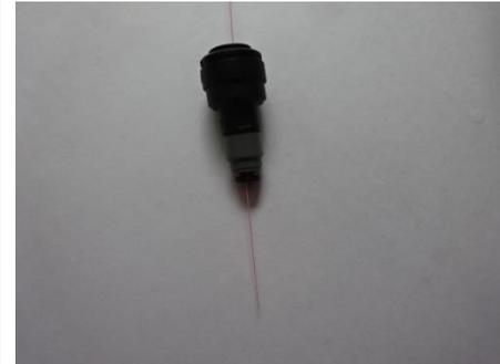
Pass the optical fibre through the 6mm – 3mm connector.
