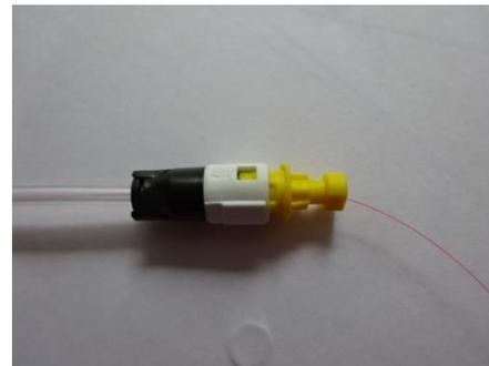
Attach the connector onto the locking tube.
