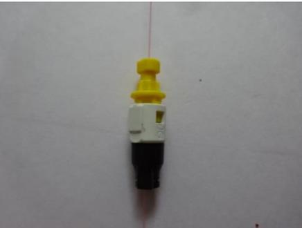
Pass the optical fibre through the connector
