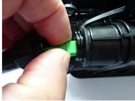
Push SC connector into the adapter. Ensure locating the rib is facing upwards to line on top of the port.
