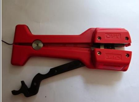
Open the cutter by pulling down on the black arm.
