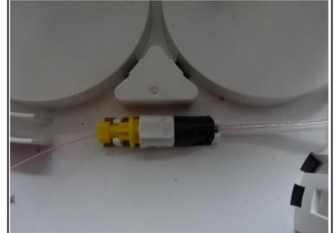
Fit the connector into the locking clips.
