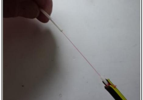
Remove the final section of the loose tube.
