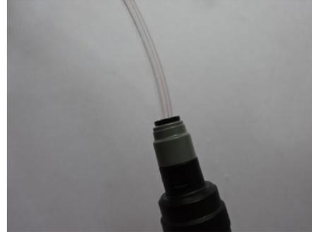
Fit the tube to the reducing connector.
