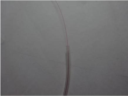
Insert optical fibre through the locking tube.
