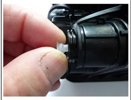
Remove the adapter blanking plug.
