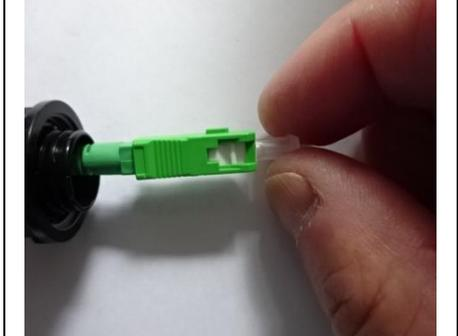
Remove the SC connector protective shroud.
