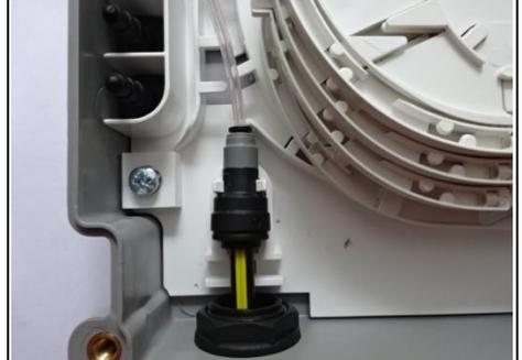
Locate the completed tube assembly into position and clip the connector into place.
