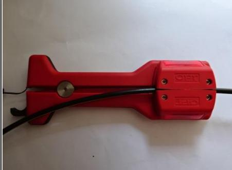
Assemble the cutter around the cable at the mark made in step 24. The blades should be positioned over the groove and yellow line.
