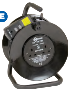
E) Heavy Duty 240V 16 amp 25 metre reel supplied with fitted RCD adaptor with 30mA trip current. Features 2 sockets.
