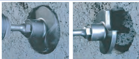
Circular cutter produces a flat back hole... ..and also pre-drills the fixing hole
